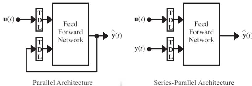
Fig1. Parallel and Series-Parallel Structures
