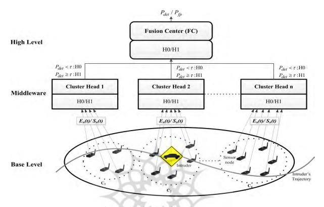
Figure 1. Architecture of intrusion detector
