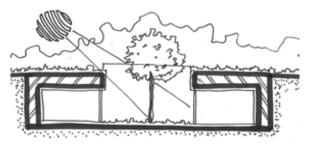
Fig.3: Bellow ground Earth-Sheltered structures
