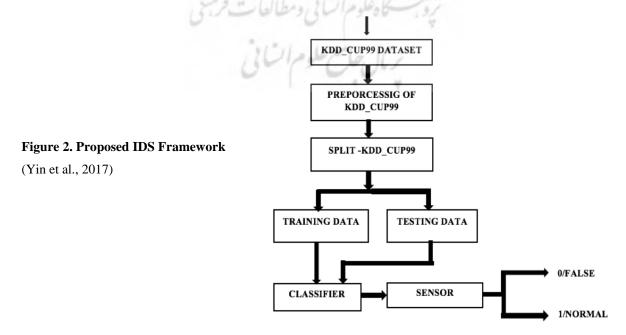
Figure 2 shows proposed IDS framework for the operation of a machine learning algorithms with intrusion detection where KDD Cup 99 dataset is observed to generate classifiers from dataset training and testing. These classifiers generate sensor result as false or normal values.
